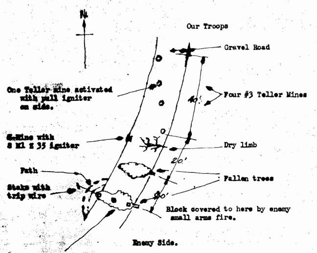
Three prepared charge booby traps with ZZ 42 igniters. Two are wired to branches to prevent stepping over trunks or moving trees from road without detention.
